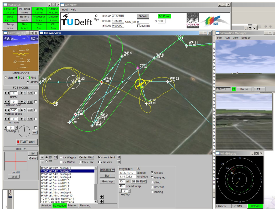
Figure 9: Ground Control Station containing the Instruments window showing flight data and FCS control modes, the Mission view with the map which is the heart of the control interface, FCS status window, the simulation manager, wind display and simulated camera view and the GCS window showing status information about the differential GPS connected to the ground control station.
